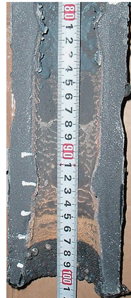
Fig. 12 Cut section of “Mogul with reverse-taper port” SEN.
