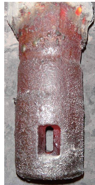
Fig. 7 Appearance of “Bend port” SEN after use.
