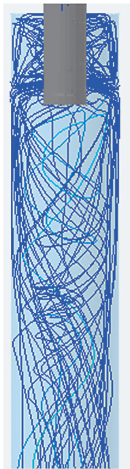
Fig. 6 CFD-calculated streamline for “Bend port” SEN.
